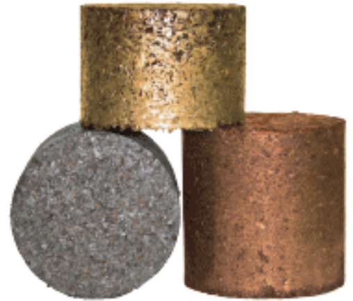
Briquettes provide a degree of quality control to recyclers that is not possible with loose chips and other swarf.
