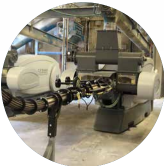
Two BP5510 briquetting presses producing industrial briquettes from softwood shavings.
